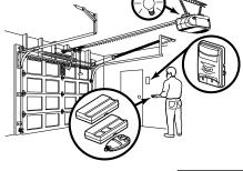
Press and release the "learn" button on the motor unit. The learn indicator light will glow steadily for 30 seconds.
